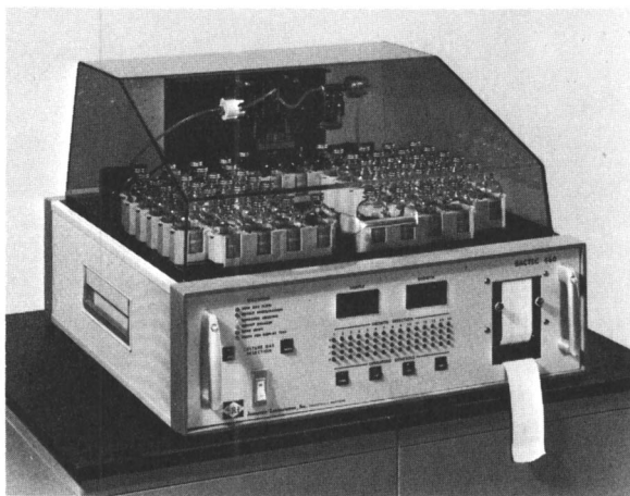
Figure 1. BACTEC model 460; an automated ionization chamber, which samples and records the amount of ^{14}\text{CO}_2 produced at a rate of one sample per minute.
